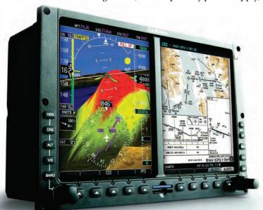
data connectivity. Class 1 EFB systems can be used both on the ground and during flight, but must be stowed for takeoff and landing. They are limited to providing supplemental information and cannot replace any required system or equipment. A Class 1 EFB may be connected to aircraft power through a certified power source to operate the EFB and recharge its batteries. A Class 1 EFB can display tabular data, such as performance tables, checklists, and the pilot operating handbook (POH).
